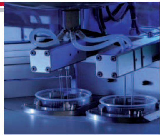
station 2 dispensing nutrient medium from a Teflon container directly to cups
