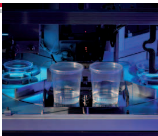
station 4 forcing closed cups out and pushing them into the area outside the dispenser
